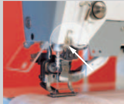
Thread monitor with optical sensor
