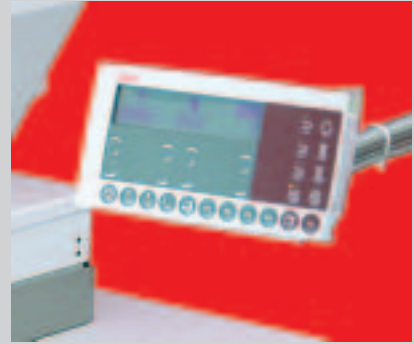
New S3 control panel with integrated data reader (SD-card) for importing sewing programs or machine software
