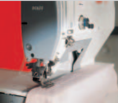
Off-set arm for easy placing/handling of workpiece
